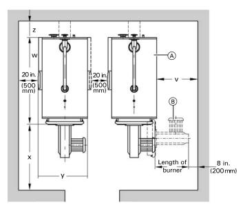
To enable convenient installation and maintenance, observe the stated clearance dimensions. Maintain the minimum clearances where space is tight. In the factory set condition, the boiler door opens to the right. You can relocate the hinge bolts so that the door can open to the left.
