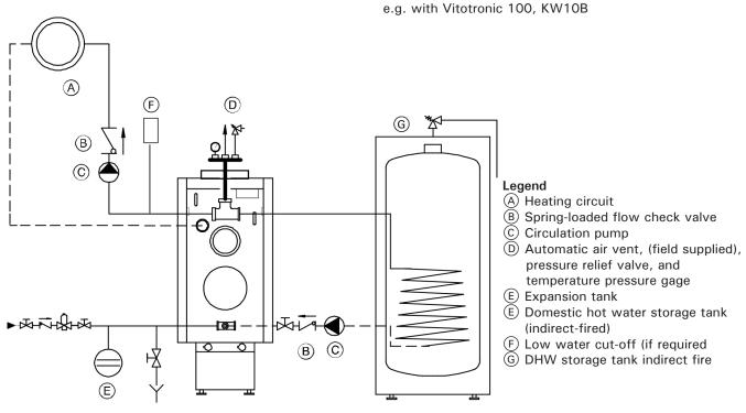
Without mixing valve and with DHW
