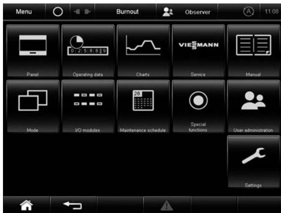
The “Menu” screen gives you access to further screens with a variety of functions. Tapping the key opens the associated screen. The functions are described in various sections of these instructions.
