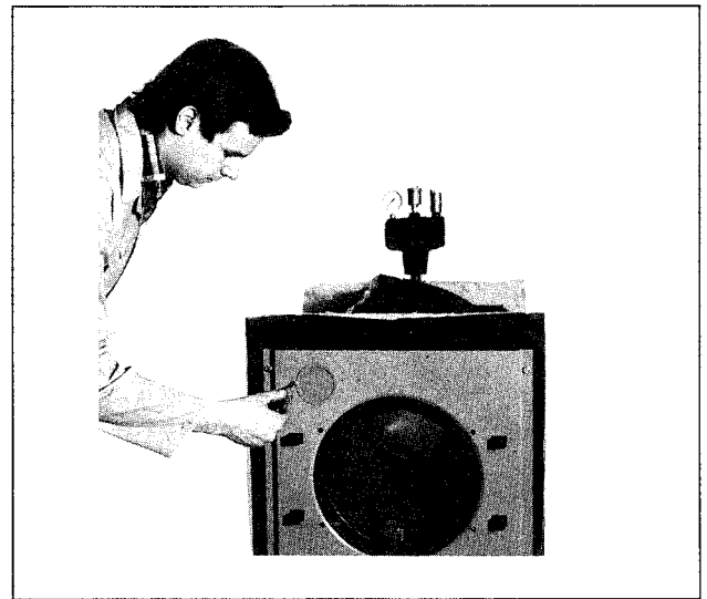
Remove cover plate over 5-point stainless steel well.
