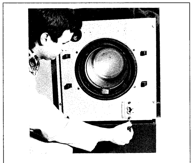
Well cover plate removed - opening wire gate.
