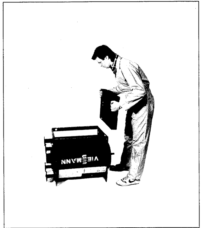
Turn boiler upside down (skids face upwards). Boiler stand front and rear panels are alike.
