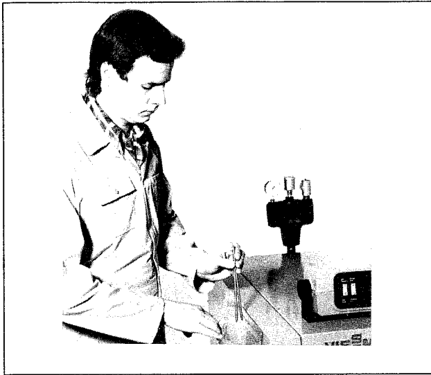
Storing of 2 spacer rods in service pocket.
