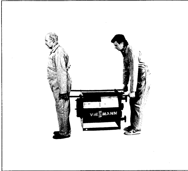
The boiler shell may be handled by a single person by means of a fridge cart, or carried by two people using 3/4" steel pipe through the lifting lugs.
