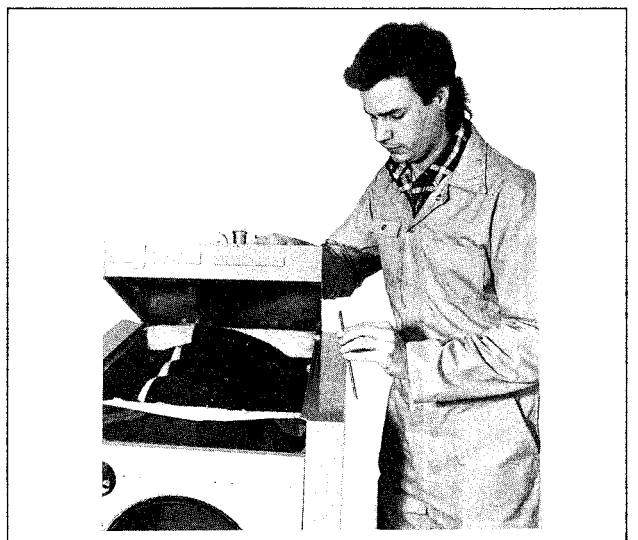
As installation help, two spacer rods are factory-supplied in the service pocket - remove and use to support top enclosure panel. Panel is secured in the back by the safety header.
