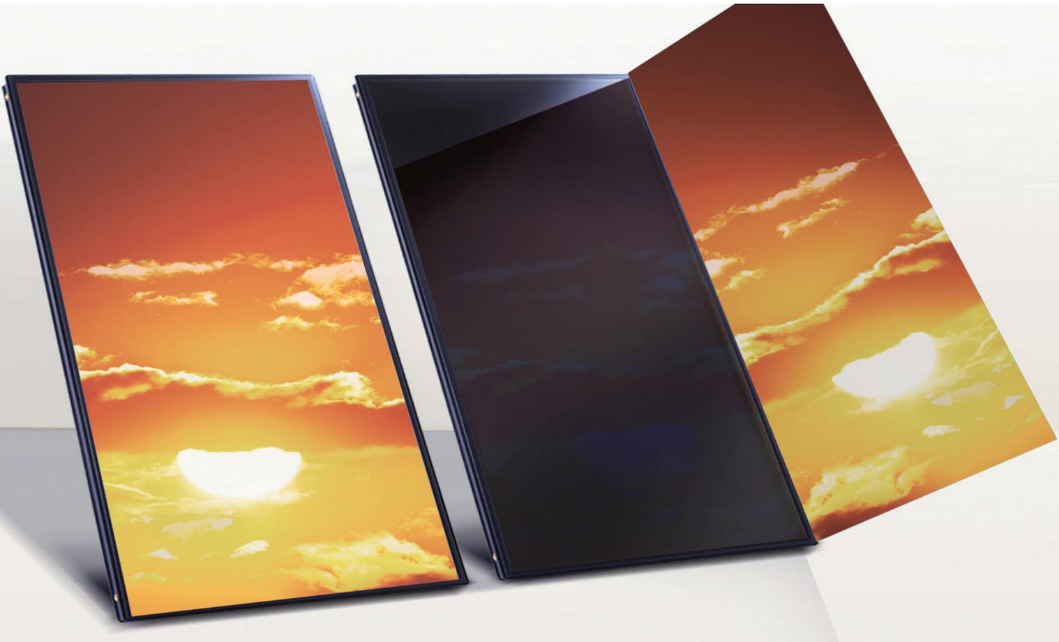
High solar coverage rates that bring substantial energy savings usually require large-scale collector surfaces. However, on warm summer days in particular, large collector surface areas can lead to long stagnation periods which causes steam formation, as the heat cannot be used. In order to prevent this steam formation, the flat-plate collectors Vitosol 200-FM and Vitosol 100-FM are now equipped with a self-regulating absorber coating.
