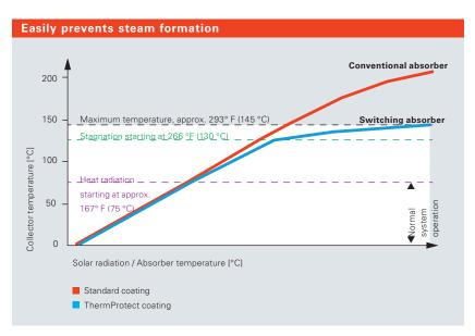
During normal collector operation, the new absorber coating of the Vitosol 200-FM and Vitosol 100-FM flat-plate collectors acts like any standard absorber coating.
