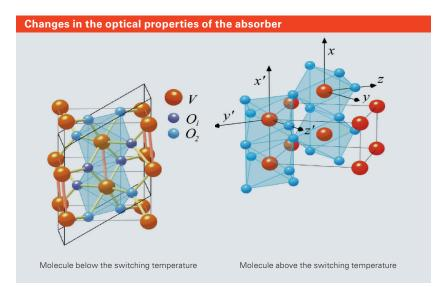
The new absorber coating consists of multiple layers. Vanadium dioxide (VO2) is one of these layers. The optical properties of Vanadium dioxide change at temperatures above the switching temperature. It heats up and thus increases the rate of heat radiation. By increasing the rate of heat emission, the stagnation temperature of the collector is reduced. The more the absorber layer heats up, the greater the heat radiation.
