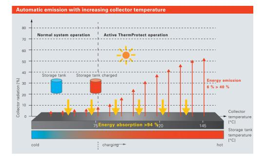
At temperatures up to the switching temperature, around six percent of incoming solar radiation is emitted. Beyond that, the heat emission automatically adjusts to a value of more than 40 percent.
