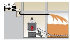
Basement storage with pellet auger
