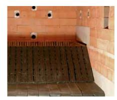
Firebrick-lined combustion chamber with external grate and moving annealing grate.
