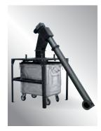
Ash removal auger and external ash container
