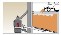
Bunker with rotary sweep extraction
