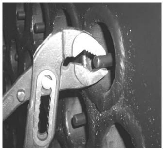
Remove the displacement rods with a pair of pliers, as shown above. The heat exchanger should be cleaned at the intervals prescribed so that performance and efficiency are maintained and the displacement rods can be easily removed.
