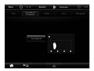
If you tap the "Secondary air/Primary air" key in the default display, the following screen is shown.
