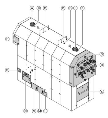
The Vitoflex 300-UF is a fully automatic solid fuel boiler with grate combustion.
