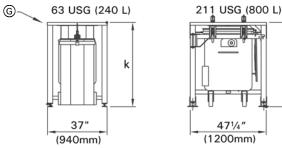
Ash bin support frame: positioning is possible in  $4 \times 90^{\circ}$  (extraction, ash container) Drawn with extraction to the right
