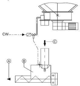
Note: A slide valve is required as standard for an unpressurized material store or a rotary valve for a material storage with overpressure or underpressure (charging with blower, e.g. wood processing operations).
